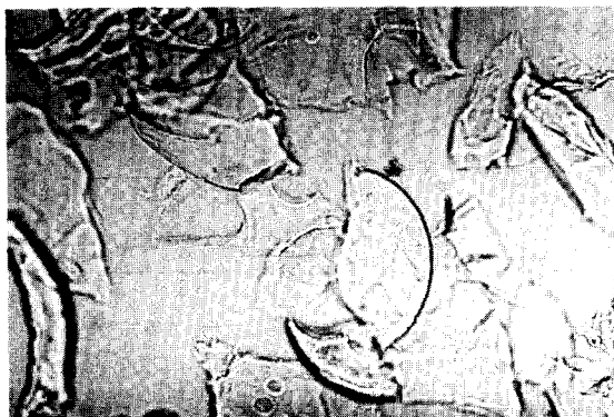
Fig. 6. Optical micrograph of ground Granocel-8 packing granules (× 90).
